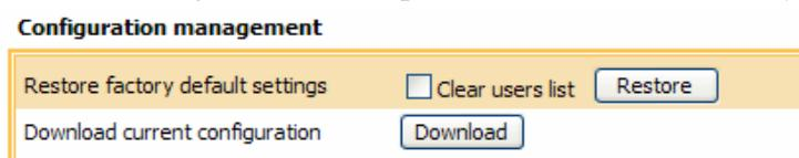
Figure 28. Restoring factory defaults settings
