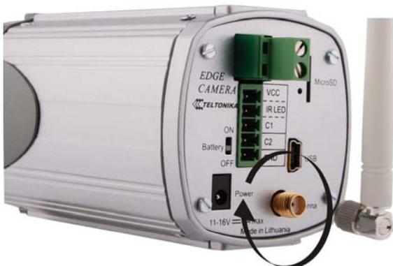
Position the antenna upwards at its connecting joint. This will ensure optimal reception.
