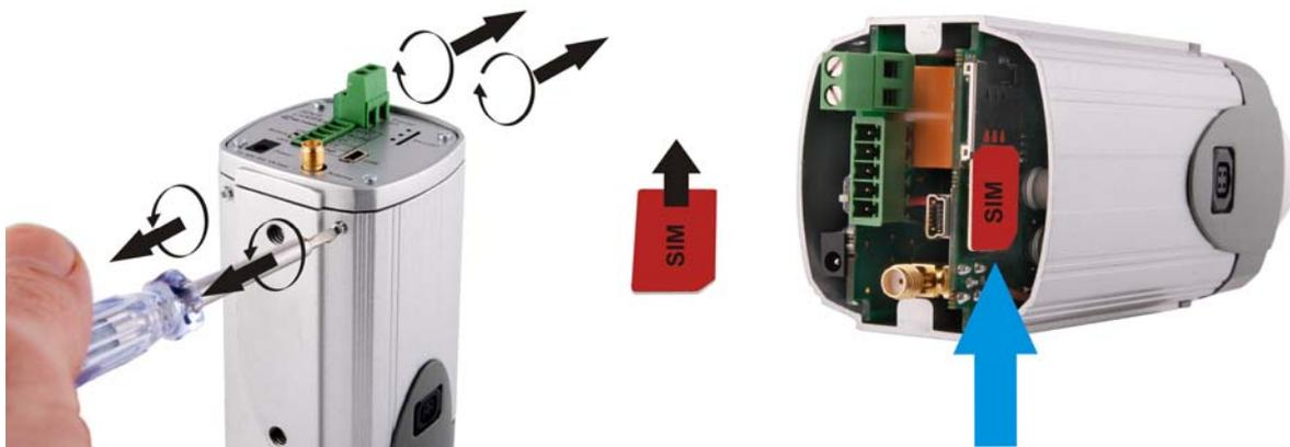
Insert the SIM card into the holder with the metal contacts facing the SIM connector side. Ensure that the 'cut-off' corner is at the bottom right as in figure above. After the SIM card is inserted attach the panel to its previous position.
