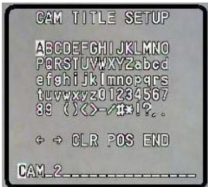
Move the joystick up or down to the desired selection.
