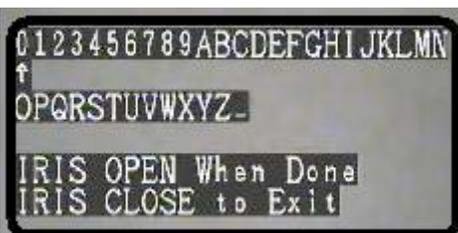
Move the joystick Left or Right to select desired character (0~9 or A~Z). Press **IRIS OPEN** button to confirm selection and move to the next character of choice.
