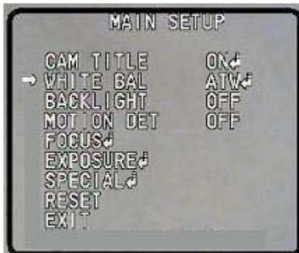
The White Balance function corrects the abnormal white color into the normal white color under any color temperature.
