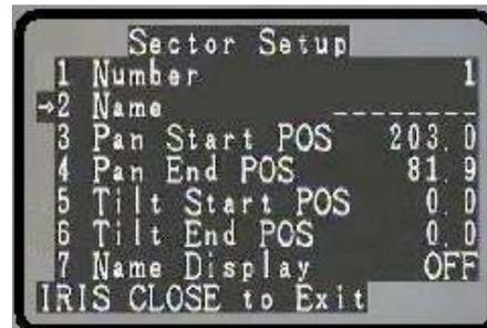
User can subsequently name the sector by moving the joystick down to the name field.
