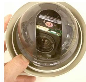
**Step 2:** Remove the camera liner to gain access to the dip switch settings located on the PC-Board underneath the camera.
