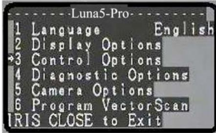
Move the joystick up or down to the desired selection.
