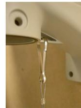
**Step 5:** Connect the end of the wiring harness protruding out of the bracket to the mating connector on the dome unit. Observe proper orientation of the connectors as illustrated.
