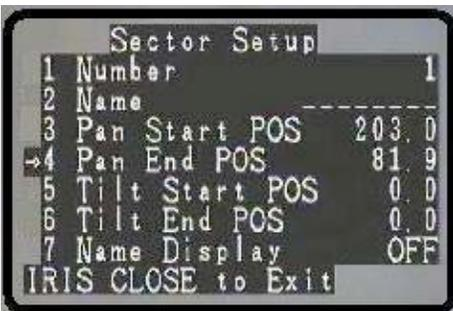
Move the joystick up or down to the desired selection.
