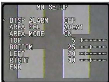
The position of the detection area can be adjusted using directional controls as illustrated. Move the joystick up or down to the desired selection.
