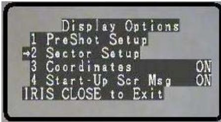
On the Display Option menu move the joystick to select the Sector Setup Menu. Confirm your selection by moving the Joystick to the right or,
