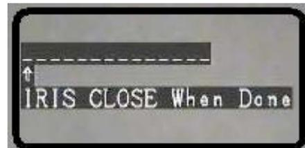
User can edit the name of a Sector position. Move the Joystick Left or Right to select desired character position and press **IRIS OPEN** button to display the character selection sub menu.
