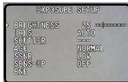
**Manual:** Shutter speed can be adjusted manually from 1/60 to 1/120000 of a second
