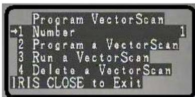
The default number is 1. Move the joystick left or right to select 1 through 6 Vectors (or tours) available. Each tour can be programmed for up to 16 preset positions with individual speed and dwell settings for each preset.
