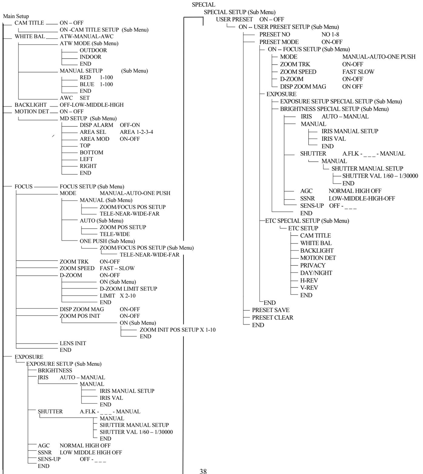
**The following section is specific to the Special Setup Sub Menu for the SAMSUNG Camera module.**
