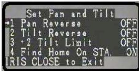
Move the joystick up or down to the desired selection.
