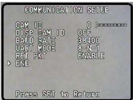
The communication parameters of the camera are factory preset and do not require any user configurations.
