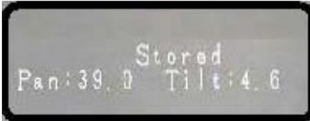
The menu will display “Stored” confirming that the position has been set in the dome memory. If you do not see the confirmation repeat the process as there may be a latency of communications depending the wiring method and the number of devices connected on the RS485 Loop.
