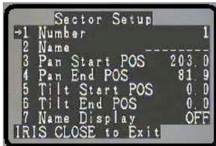
A sector is defined as a general area bound by user set coordinates on both axis (X, Y) Example: you can define North as an area bound by an arc between North-West and North-East. When the PTZ is pointed in this general area, the name North, will appear on the screen.
