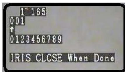
The default number is 001. Move the joystick left or right to position the cursor under the desired numeral and press **IRIS OPEN** button to move the cursor on the second numeral line (0~9). Move the Joystick left or right again under the desired numeral and press **IRIS OPEN** button again to select the desired number (0~9). Press **IRIS OPEN** button again to confirm the selection. Press **IRIS CLOSE** button to finalize your selection and return to the previous menu level.
