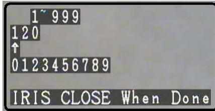
The default number is 120 seconds. This is the time delay before the PTZ returns to the default position after 120 seconds of inactivity.
