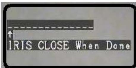
User can edit the name of a preset position. Move the Joystick Left or Right to select desired character position and press **IRIS OPEN** button to display the character selection sub menu.
