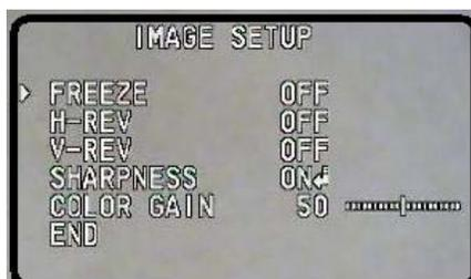
For specific placements of the Dome unit such as upside down or specific circumstances, the user has the ability to adjust the image such as Horizontal and Vertical flip, modify the Sharpness, and color gain.
