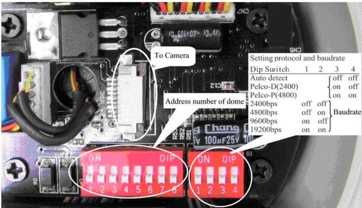
Note: The illustration shows the two Dip-Switches. The switch on the left (8 position) is for the dome address while the switch on the right is for the protocol and baudrate settings.
