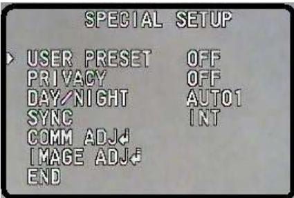
Under USER PRESET the user can select a variety of options related to the specific behavior of the camera regarding Focus, Exposure, White Balance and others features for specific preset settings, There are a total of 8 positions that are user configurable in great detail.
