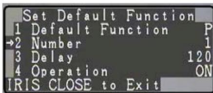
The default number is 001. Move the joystick left or right to position the cursor under the desired numeral and press **IRIS OPEN** button to move the cursor on the second numeral line (0~9). Move the Joystick left or right again under the desired numeral and press **IRIS OPEN** button again to select the desired number (0~9). Press **IRIS OPEN** button again to confirm the selection. Press **IRIS CLOSE** button to finalize your selection and return to the previous menu level.
