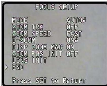
**ZOOM TRACK:** When it is turned ON the focus function is executed when the zoom function is ON. **SPEED-FAST** will speed up the ZOOM, Slow has the opposite effect.
