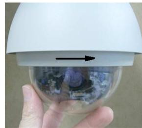
**Fig. 18** Rotate clockwise as indicated
