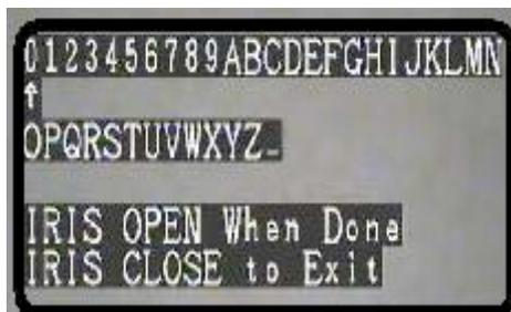
Move the joystick Left or Right to select desired character (0~9 or A~Z). Press **IRIS OPEN** button to confirm selection and move to the next character of choice. Press **IRIS CLOSE** button to exit or return to the previous menu level when programming is done.
