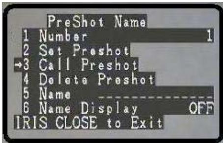
Based on the displayed/selected preset position on line 1 of this menu, the dome will respond upon moving the joystick to the Right position and position itself to the corresponding coordinates (X,Y, Z) of the selected preset position.
