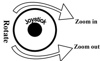
The operation of the dome and the direction (up, down, left and right) of the camera can be controlled using the joystick of the keyboard controller, as illustrated above.
