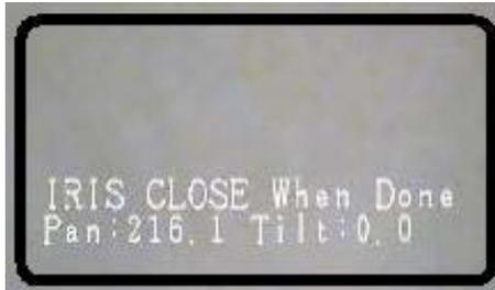
Move the Dome camera to the desired position on all 3 axis (P,T,Z) and then press **IRIS CLOSE** button to confirm the preset position location and return to the previous menu.
