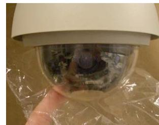
**Fig. 19** Protection film of acrylic shield
