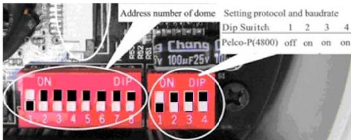
This illustration demonstrates the settings for Dome Address 1, with Protocol Pelco -P at a baud-rate of 4800 setting.
