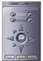
: PTZ cameras connected to VC DVR DVR System can be controlled from VC DVR Net. The arrow buttons will move the camera in the direction of the arrow, and the ZOOM, FOCUS buttons will manipulate the camera accordingly. However, only user with permission can control the PTZ setting.
