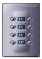
: Adjusts the image quality such as Brightness, Contrast, Saturation and Hue by pushing the arrow buttons.
