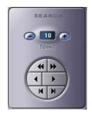
: Buttons in upper line works for fast rewind (left directional arrow) and fast forward (right directional arrow). Buttons in middle line activate the normal playing back in forward and reverse but the speed can be adjusted by controlling ( - ),( + ) tap on the top. The buttons in lower line give playback frame by frame, forward or reverse.
