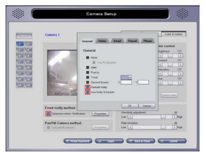
From "Color & motion" of "Camera Setup", check "Detective motion – Notification". Click on "Properties", and check "Remote Notify" to send notifications when an event occurs. Check "Use Notify Schedule" to utilize the schedule to notify the VC DVR Net. If selected, notification schesule on the folloing page must be configured.
