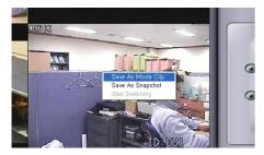
**Save as Movie Clip:** check to create mp4 format movie clip until unchecked. Recording will be automatically finished when Net software is minimized. Recorded file will be stored at the location assigned from MISC. Configuration, AVI Path.
