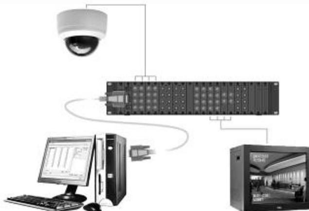
Note: With a view to enabling users to generate character, our company provides the Compact Disk with character generating software on it. You could connect it with PC through the serial port line, and then use the software to generate character. That could make things much easier – eliminating the process of looking up complicated Character Table.
