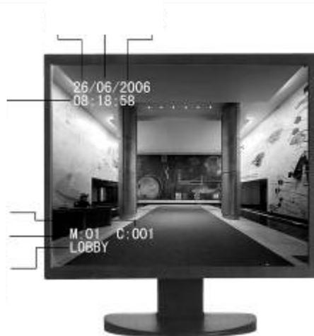
When the system is electrified, the image standard displayed on the monitor will be: Time is showed in the upper right hand side, character of current camera description, camera number and the monitor number can be found in the bottom left corner. Pls refer to **operation manual for VC-SC1000M controlling keyboard** for its general operating method. Other special operation are as follows:
