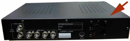
**STEP 1. REMOVE THE 3 SREWS AS FOLLOWINGS FROM THE REAR SITE AND OPEN THE UPPER COVER**
