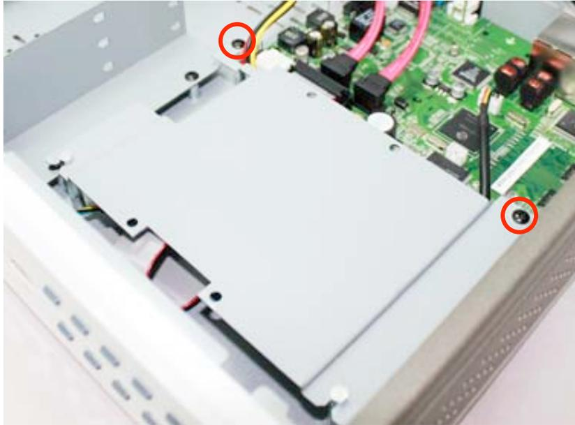
**Step 4** Slide the bracket slightly backwards and then lift it out.
