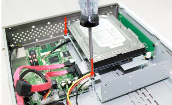
**Step 8** Attached the hard drive data cable and power cable to the hard drive.
