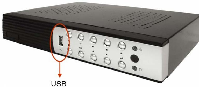
You can change the time period of recorded data for backup by setting the “Start Time” and “End Time” and plug in the USB disk.
