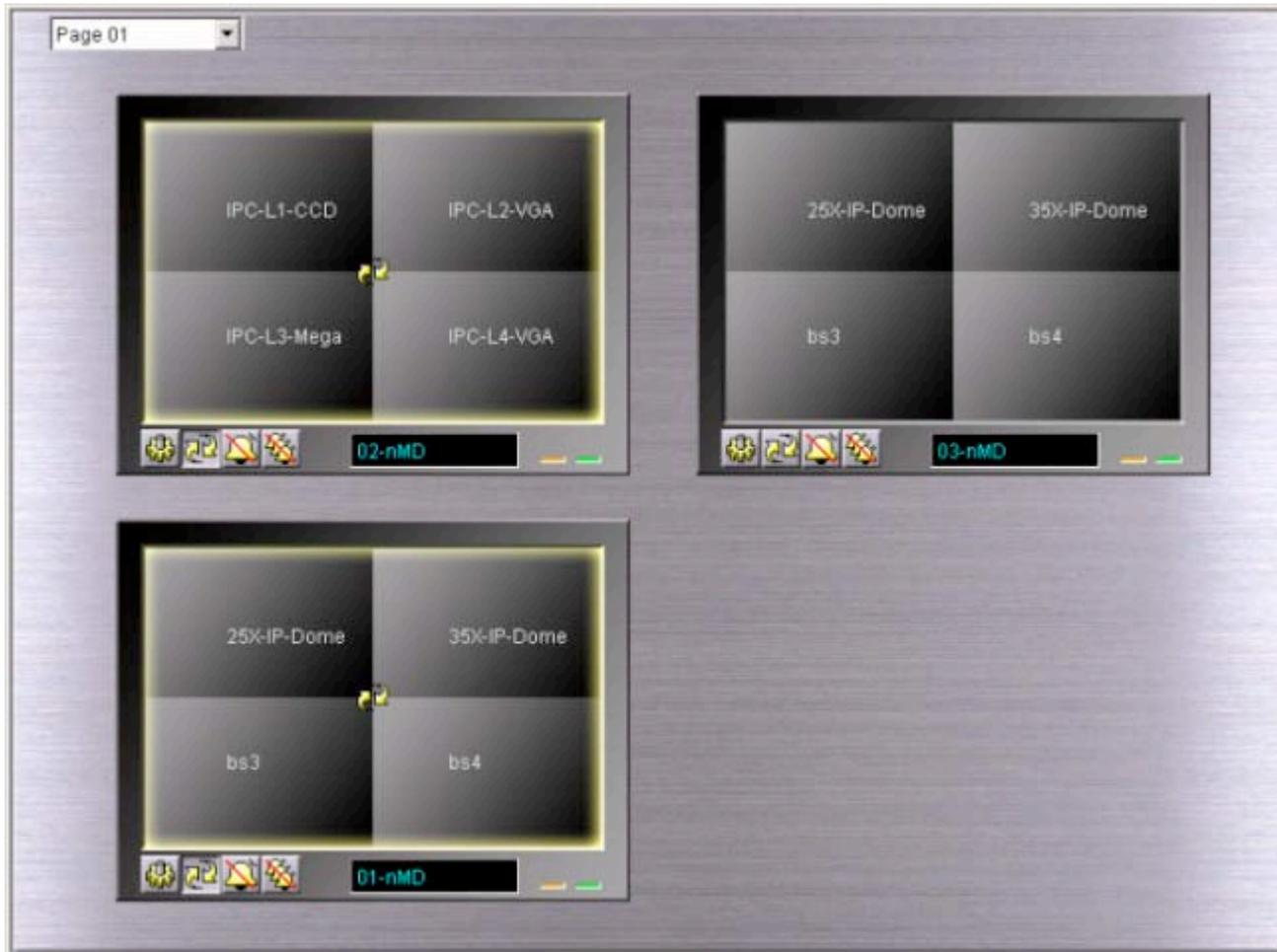
**Monitor** helps you to setup the **Video Wall** or **Video Matrix** with the monitor output devices auto-detect by the CMS server. Each Video Decoder has up to quad-screen display. With the **Sequence** display function, it could display up to 64 cameras.
