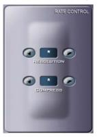
: Compression Rate can be adjusted between 10  $\sim$  90 to enhance the transmission speed (\* for default compression rate). Lower value will provide faster transmission. Resolution can be selected among 1/2, 1/4, or 1/8 (\* for default resolution), and lower resolution provides faster transmission speed. Compression rate and resolution adjusted here are not changing actual resolution and compression rate recorded on the server.
