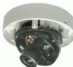
Open dome with board camera and DC-vario lens
