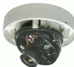
Open dome with board camera and lens
