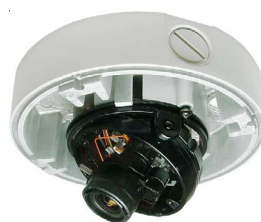
Open dome with board camera and DC vario lens
