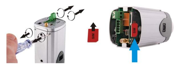
Insert the SIM card into the holder with the metal contacts facing the SIM connector side. Ensure that the 'cut-off' corner is at the bottom right as in figure above. After the SIM card is inserted attach the panel to its previous position.
