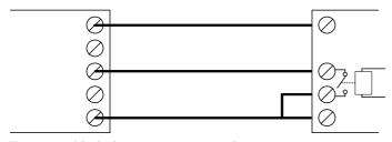
Figure 29. Typical PIR sensor connection
