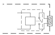
Figure 2. Internal camera relay connected to 2-pin terminal block.
