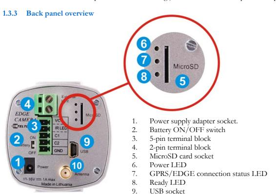
Figure 1. EDGE camera back panel view.
