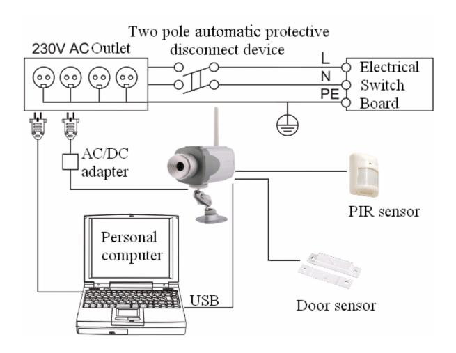
Protection against over currents, short circuits and earth faults an additional two-pole disconnect device shall be provided as a part of building installation. This protection device shall have adequate breaking capacity to interrupt the maximum fault current which can flow and shall have a contact separation of at least 3 mm.
