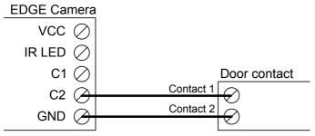
Figure 30. Typical magnetic door sensor connection
