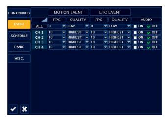
When event triggered, you can configure recording condition like follows;
