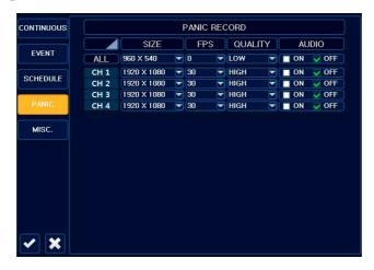
During panic recording mode, the MV8004S will override all other recording settings and record continuously on all channels at the settings configured here.
