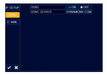
**♣** DDNS: When enabled the MV8004S can be accessed through a <u>dynamic DNS server</u>. Commonly used if a broadband connection does not have a static IP address.
