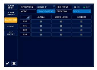
You can configure Buzzer output when event triggered.
