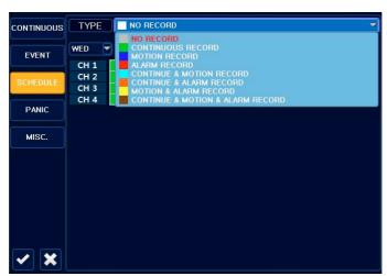
You can configure schedule time table using left mouse click or Front key (press event key button and use arrow key for top/bottom/left right. And you can press the enter key twice at Front panel to select one block.
