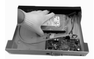
3. Place the HDD in accordance with the four holes in the bottom.
