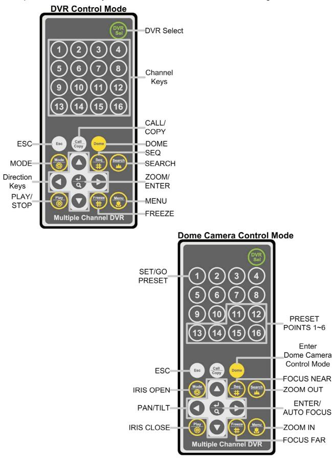
The keys of the remote control function as the keys of the front panel of the DVR. The only difference between the remote control and the front panel keys is the "DVR SEL" key. The DVR Selection key is used to switch control between each DVR.
