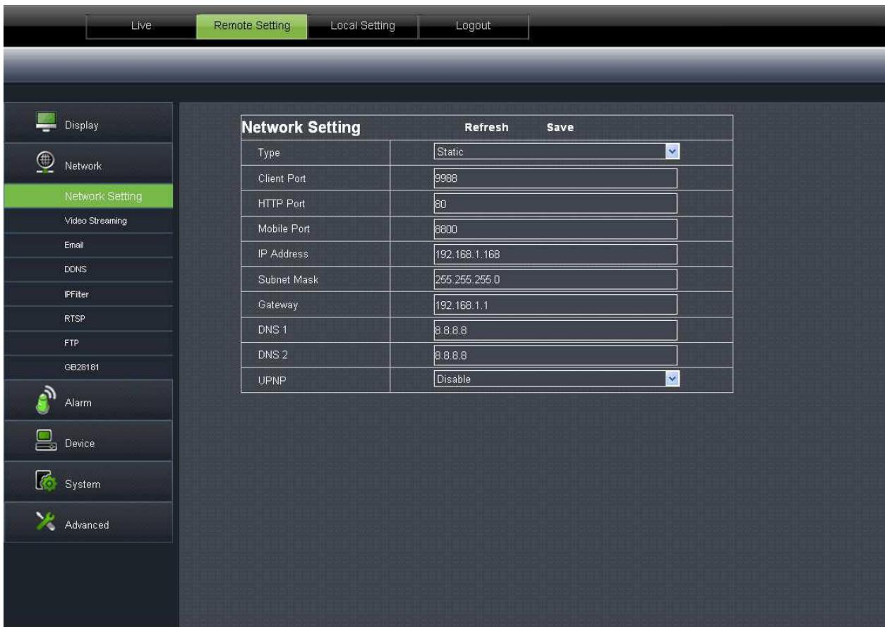
Type: DHCP or Static. Default type is Static.
