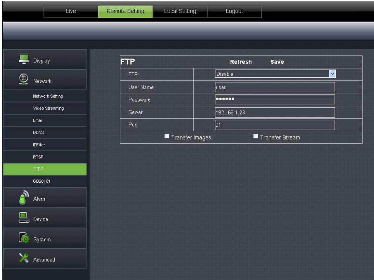
**FTP** : FTP service setting. This function is applied together with alarming function. The captured images or alarming recording can be uploaded to FTP server through network.
