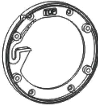
Step 4 Hang the integrated camera into the base along the guide slots and rotate it to a certain angle to facilitate cable connection, as shown in Figure 3-3.
