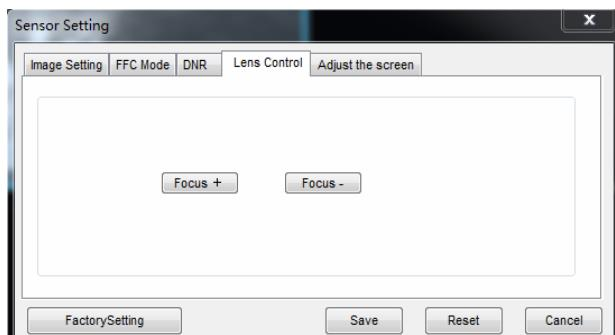
This interface is used to control focal distance of electrically-controlled lens.
